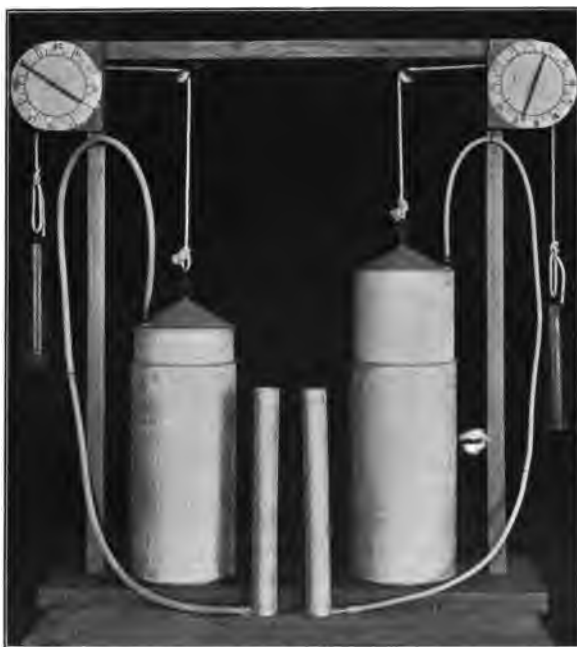
FIG. 56. Aspirator for determining the Rate of Movement of Air through Soils. (Adapted from Bul. 107, U. S. Dept. Agr., Office of Expt. Stations.)
